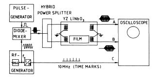
FIG. 2. Block diagram of electronics for the SAW measurement.
