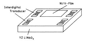
FIG. 1. Geometrical arrangement of transducers and superlattice on the LiNbO<sub>3</sub> substrate.
